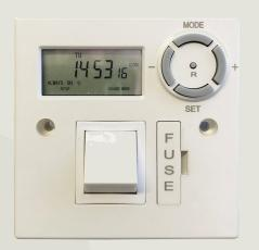
OP-DFST IS A DIGITAL FUSED-SPUR TIME SWITCH. THE TIMER IS SUITABLE FOR PATRESS BOX MOUNTING. THE 7 DAY PROGRAMMING LOGIC CONTROLS A MAINS-LINKED SWITCH, WITH A RESISTIVE RATING OF 13 AMPERES. THERE IS AN INBUILT RE-CHARGEABLE CELL TO KEEP THE TIMER RUNNING IN THE EVENT OF A LOSS OF MAINS POWER. THE OUTPUT CAN BE DISCONNECTED BY AN INTEGRATED DOUBLE-POLE ISOLATOR SWITCH; THE LOAD IS PROTECTED BY A REPLACEABLE BS1362 13 AMPERE CARTRIDGE FUSE, WITHIN A REMOVEABLE CADDY.
